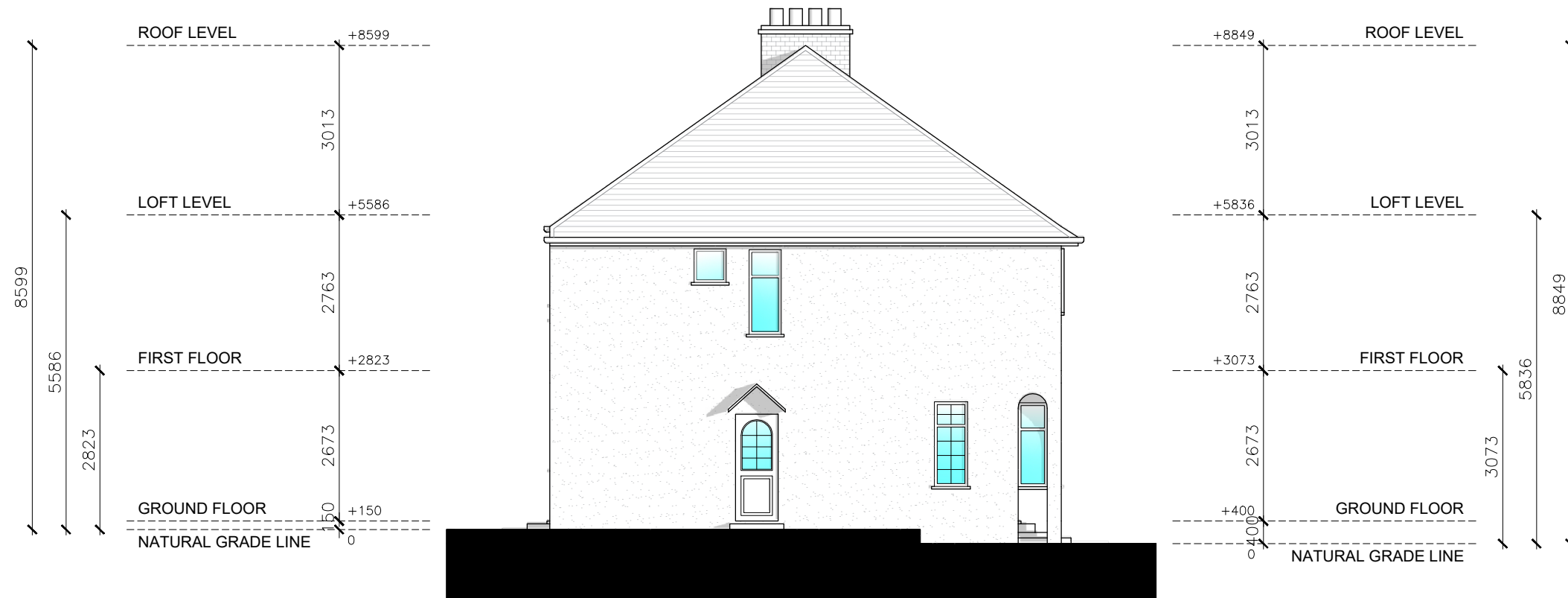
SOUTH-EAST ELEVATION (LEFT SIDE VIEW)
