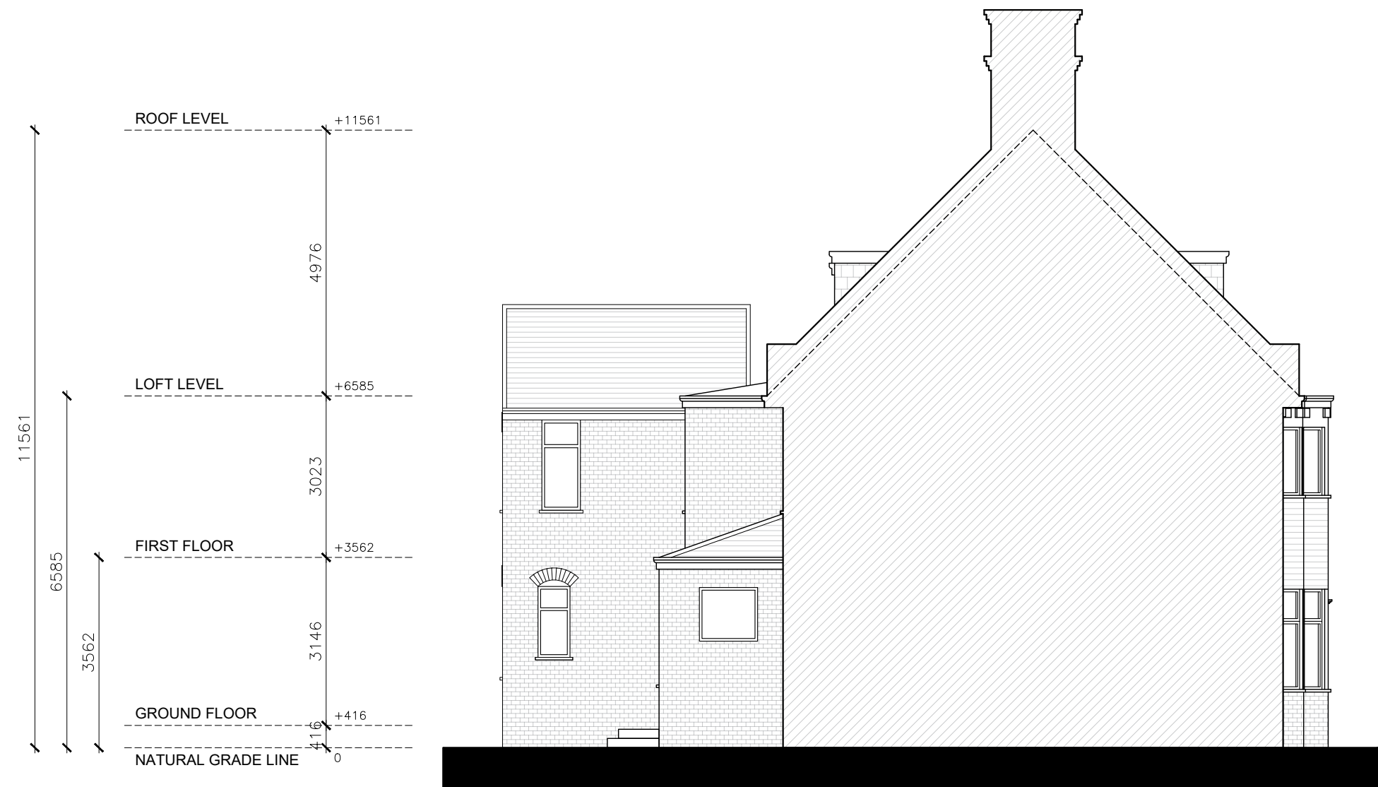
SOUTH-EAST ELEVATION (LEFT SIDE VIEW)
